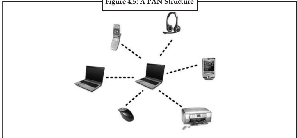
Figure 4.5: A PAN Structure
